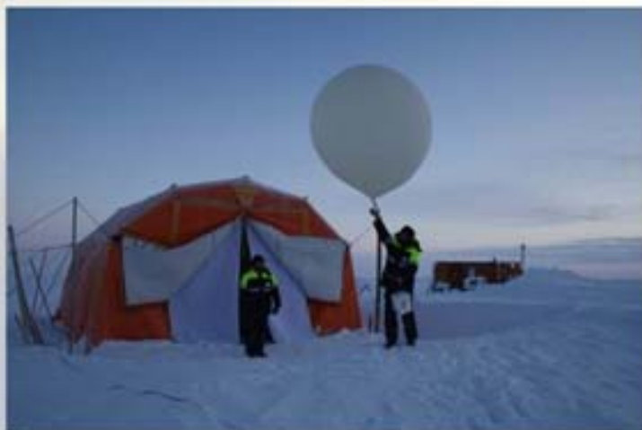
Launching of ozone sound at drifting station “North Pole 38”
