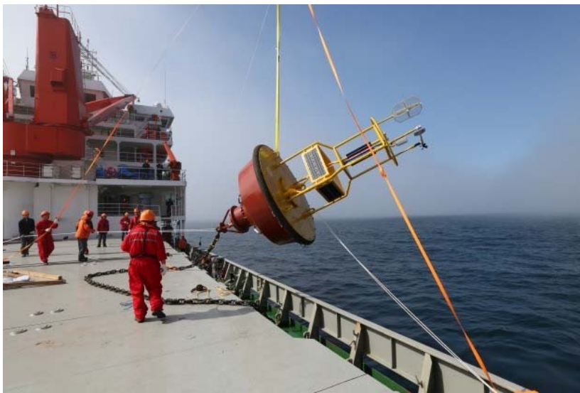
air-ocean flux mooring system
