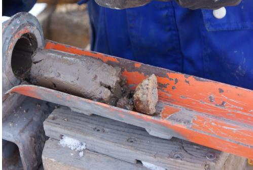
Example of Cores collected at CCT borehole between the ground surface and 3.7 m of depth
