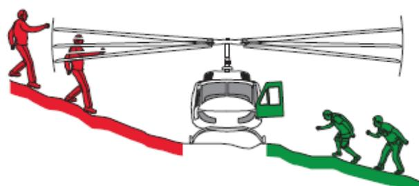
Figure 4.2 Correct and safe behaviour for helicopter operations.
