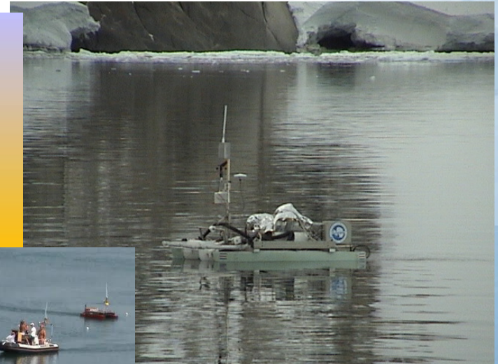
Charlie USV sampling the surface micro-layer and immediate sub-surface water along paths specified by the scientific end-user (Tethis Bay - Antarctica)
