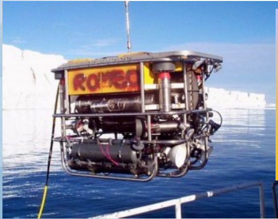
Romeo ROV ready for the exploration of the Campbell Glacier's ice tongue (Ross Sea, Antarctica)
