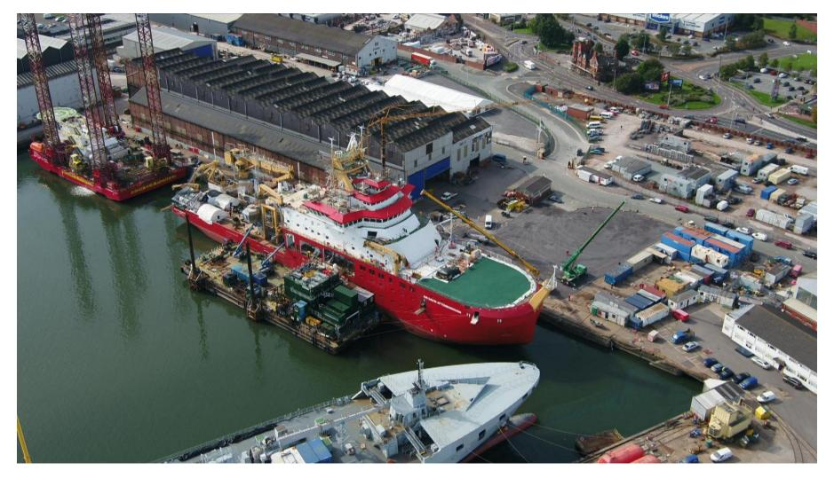
128m length, 24m beam; 15,000 gross tonnes; 900m3 scientific cargo capacity; moon pool; 60 day endurance; 60 scientists and support staff; remotely piloted instruments for deep ocean and under-ice data capture
